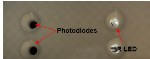
Figure 3; How the distance sensor will be setup for D-MILE to measure the height of the print bed.
